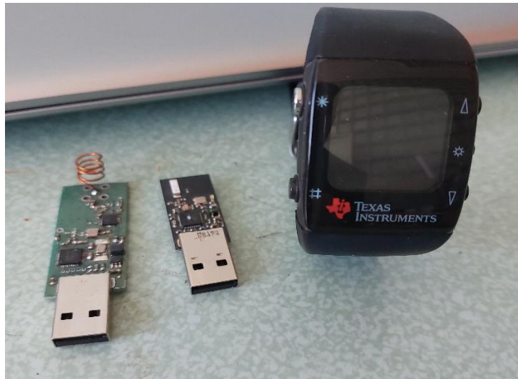
Fig. 1. Smartwatch EZ eZ430-Chronos with accessories for programming and debugging.
