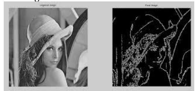
Figure 2: Example for Canny edge Detection [1]
