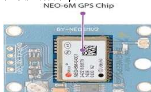
Figure 3.7 NEO-6M GPS Module
