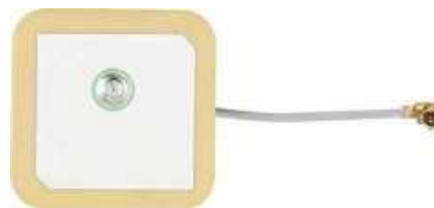
figure 3.11. NEO-6M Patch Antenna
