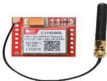
Figure 3.5 SIM800L GSM Module with 2dBi Duck
