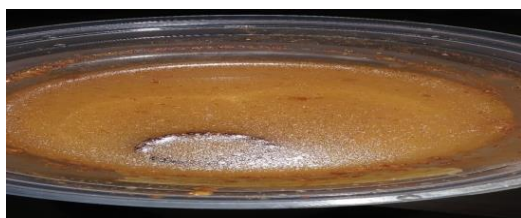
Plate 2: galvanized iron in an acid container after ten days
