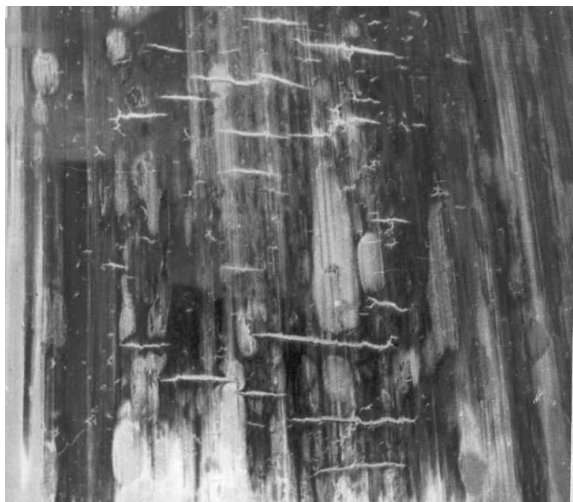
Figure 4: Brake pulley friction surface with microcracks and partial thermal spots
