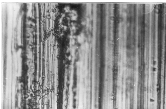
Figure 5: Brake pulley friction surface with adhering particles from the pad material Retenaks FK-24A
