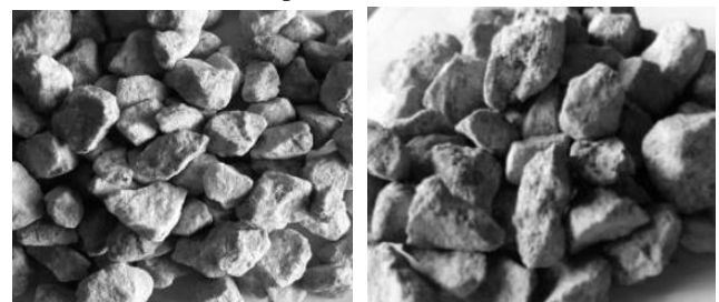
Figure 2: Natural aggregate and Crushed Concrete Waste
