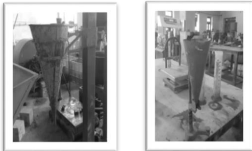
Figure 3: Marsh Cone apparatus for Cement & mortar (5mm and 12mm diameter mouth)
