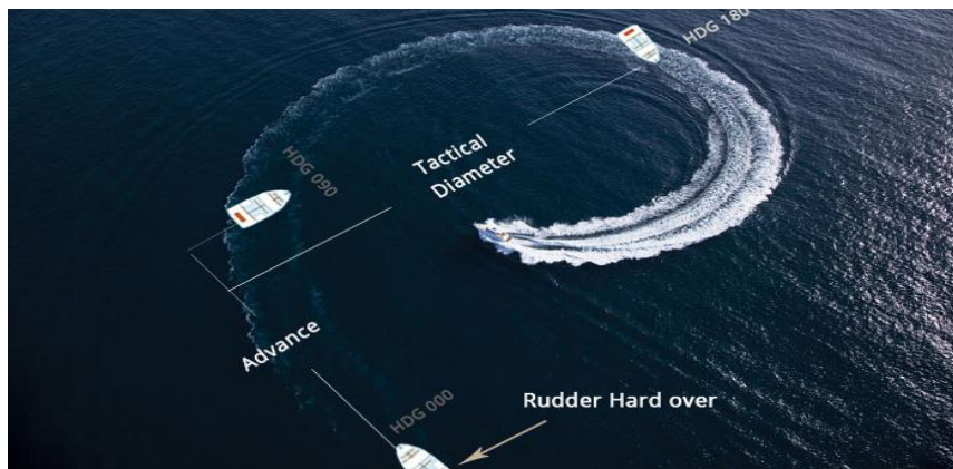
Fig. 1. Typical maneuvering test, depicted is the tactical diameter assessment between two vessels for maneuvering
