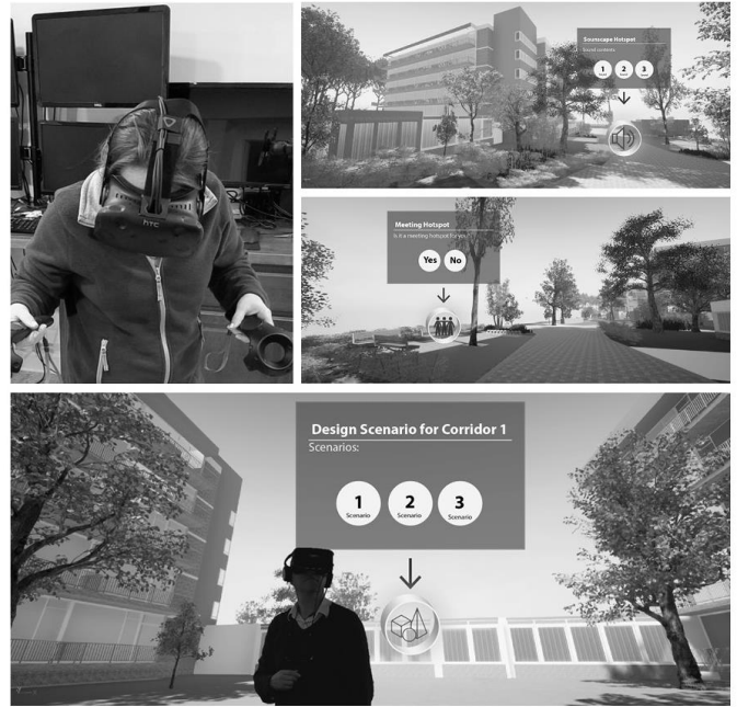
Fig. 6. The smart placemaking VR exploration of proposed design scenarios in Malvalaan neighbourhood
