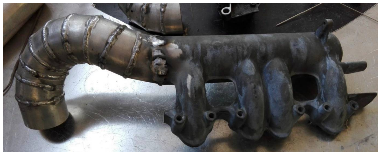
Figure 3. Intake manifold proposed for the retrofit.
