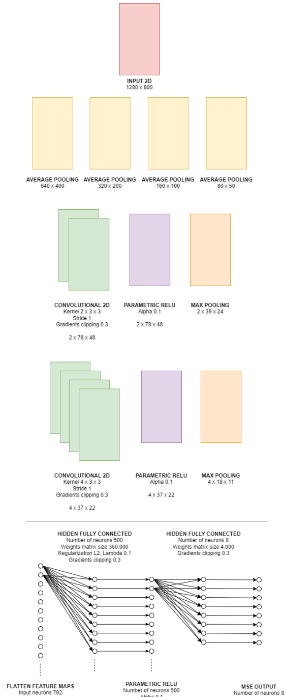
Fig. 2. Convolutional neural network for eye location
