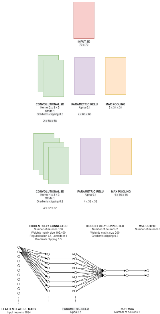
Fig. 3. Convolutional neural network for eye patch classification
