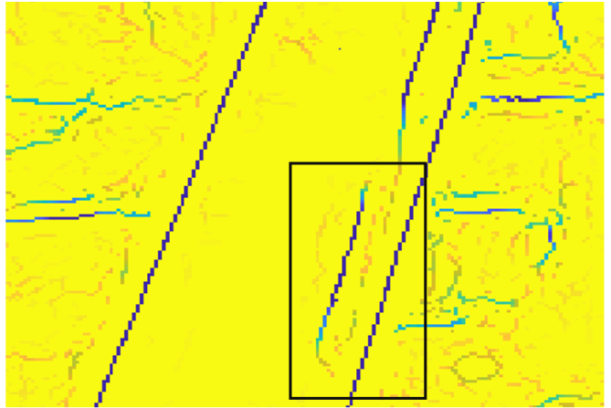
Fig. 2. Edges detected by the structural random forests. The black rectangle shows that more than one edges are detected, where only one is expected. Prominent edges are marked in dark blue, while other weak edges are marked in light colours.
