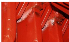
Figure 2.2 Surface PD destroys anti-corona coating
