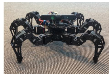
Figure.1. Hexapod Robot made by Malmros and Eriksson, 2016 [3]
