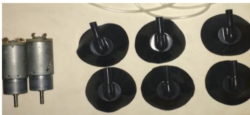
Figure.8. Six Suction Cups (Black parts) and two motors (left side) for climbing technique.
