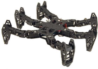
Figure.2. Aluminium structure of the intelligent Hexapod Robot [2]
