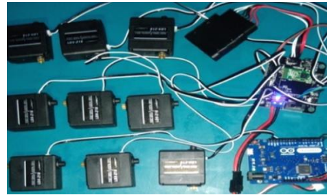
Figure.9. The mechanical throng of servo with the servo shield and microcontroller.
