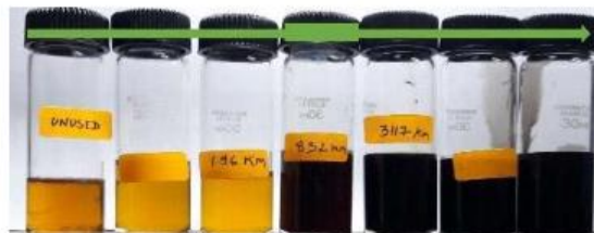
Figure 1: Degradation of oil sample after predefined interval of distance run by engine.
