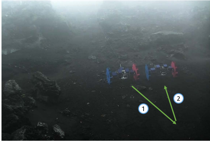
Fig. 10 Down-and-up-motion to move the robot horizontally. It proved the effectiveness of the Passive tether-guide module in a real environment.
