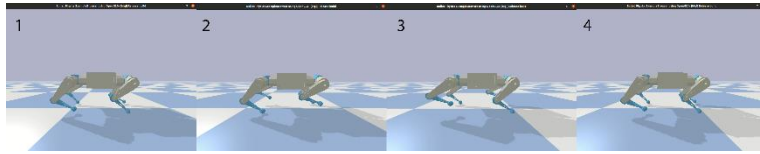
Fig. 8. Robot visualization in the PyBullet simulation environment while executing trotting gait
