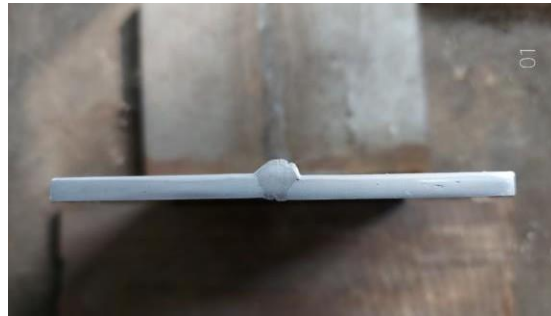
Fig. 3. Weld test piece (Etched specimen).
