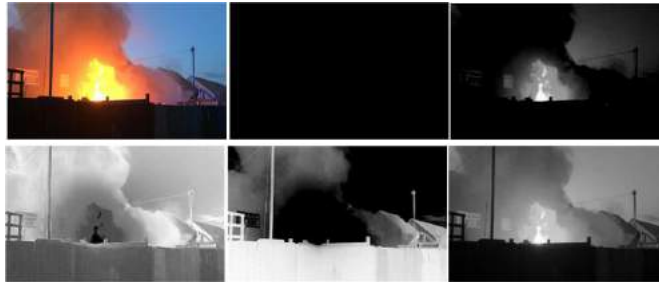
Figure 3: Five color channels generated by the color sub-network. The top left picture is the input image, and the others are the five color channels images of the output layer.
