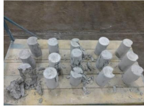
Fig. 1. Concrete specimens tested by compressive strength
