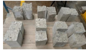
Fig. 5. Concrete specimens tested by flexural strength
