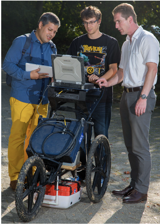
Fig. 1. The GPR hardware infrastructure.
