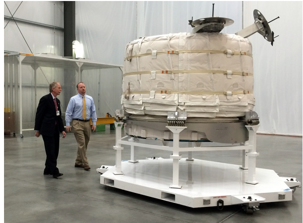
Figure 4. Undeployed BEAM Habitat at the Test Facility. Image Credit: NASA/Bigelow
