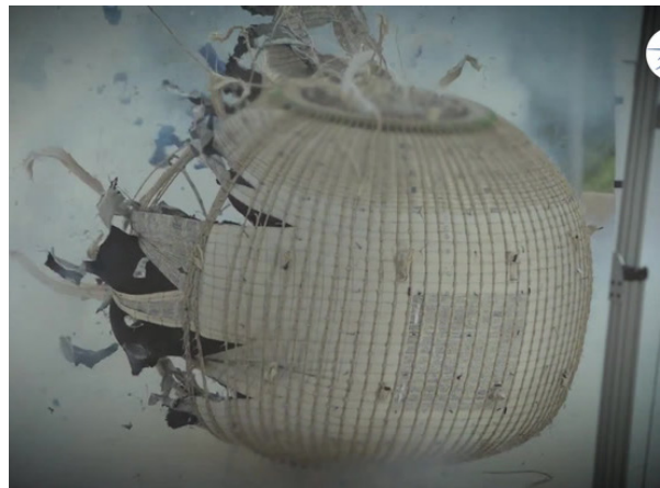
Figure 8. Lockheed Martin's Deployable habitat undergoing Burst Test (the test achieved validation by getting up to 253 psi – 6 times the maximum operating pressure). 21 Image Credit: Lockheed Martin
