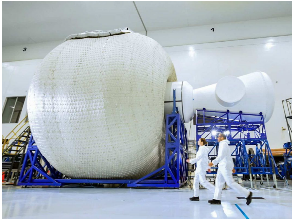
Figure 5. Fully Deployed View of LIFE Habitat. Image Credit: Sierra Nevada Corporation
