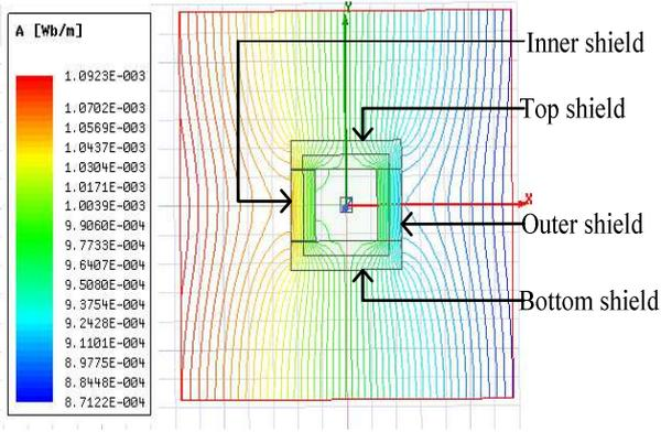
Fig.4 Magnetic field distribution for Rogowski coil with horizontal air gap for vertical external Field for a=10mm, b=10mm and g=0.2mm
