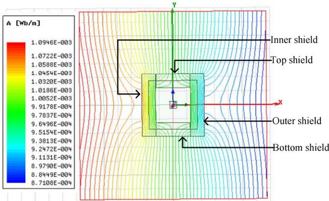
Fig.5 Magnetic field for Rogowski coil with vertical air gap for vertical external Field for a=10mm, b=10mm and g=0.2mm
