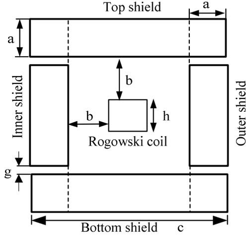
Fig.2 Magnetic circuit model with horizontal airgap
