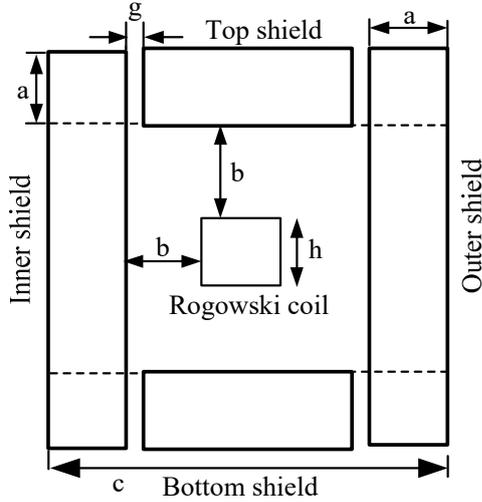
Fig.3 Magnetic circuit model with vertical airgap
