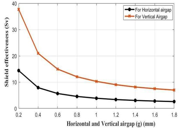
Fig.6. Relation between air gap and shield effectiveness for horizontal vertical airgap.
