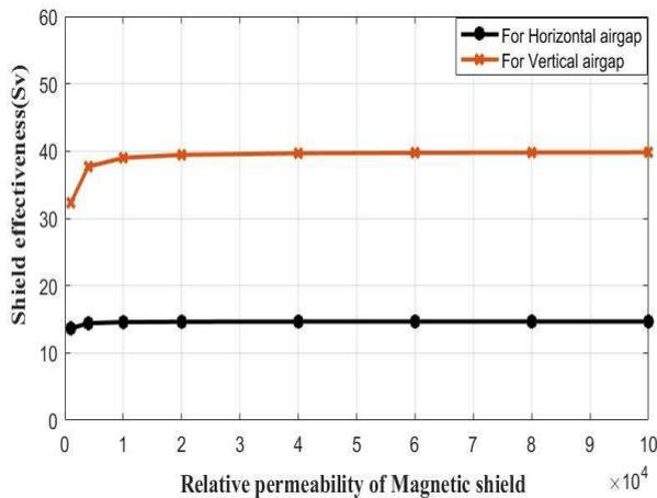
Fig.7. Relation between relative permeability of magnetic shield and shield effectiveness for horizontal and vertical air gap
