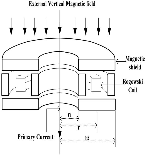
Fig. 1 cutaway view of the non-magnetic core of the Rogowski coil surrounded by the horizontal airgap of magnetic shield
