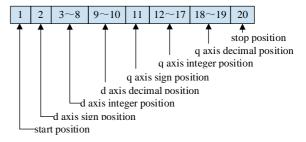
Fig. 6. Baseband signal data frame structure diagram
