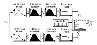
Fig. 7. Block diagram of non-coherent demodulation
