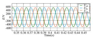
Fig. 10. Output line voltage waveform of parallel inverter
