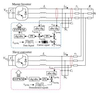
Fig. 2. Parallel inverter system structure
