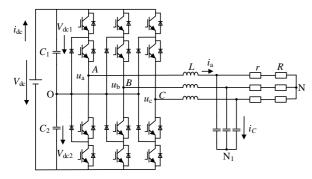
Fig. 1. Three-level three-phase bridge inverter main circuit topology
