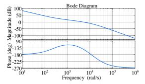
Fig. 4. Bote diagram of system open-loop transfer function
