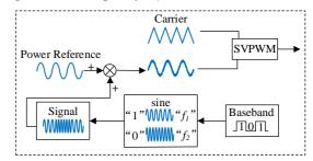
Fig. 5. Power modulation wave band modulation schematic
