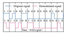
Fig. 9. The transmitted baseband signal and its corresponding demodulated signal
