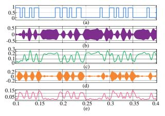
Fig. 8. Correlation waveform of power modulated waveform based signal transmission system a) baseband signal; b) "0" band signal; c) upper envelope waveform of "0" band signal; d) "1" band signal; e) upper envelope waveform of "1" band signal
