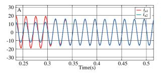
Fig. 13. Output current waveforms of parallel inverter
