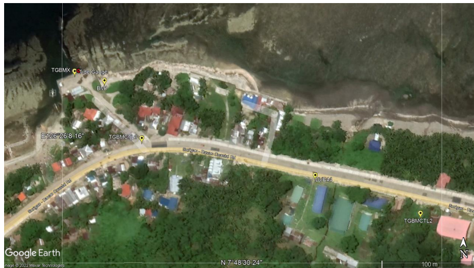
Fig. 8. Location of benchmarks used in the levelling. Yellow points are the benchmarks in reference to the location of the tide gauge (red point).
