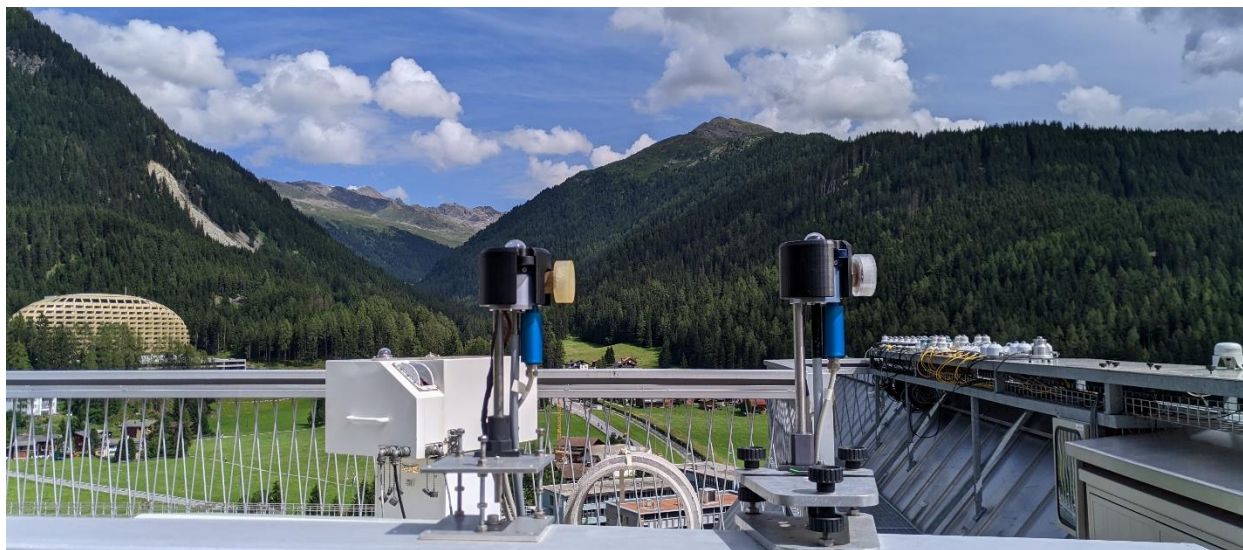
FIGURE 2. The roof platform of PMOD/WRC with the entrance optic of two reference spectroradiometers in the front and the installation of the test radiometers participating to the UVC-III in the back.
