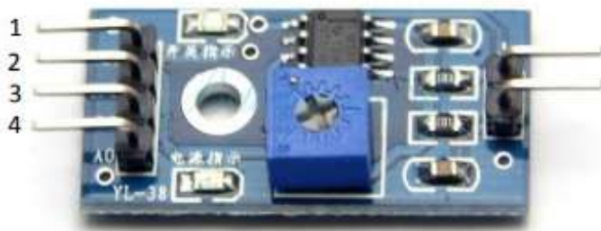
Figure 4.4 RAIN SENSOR MODULE
