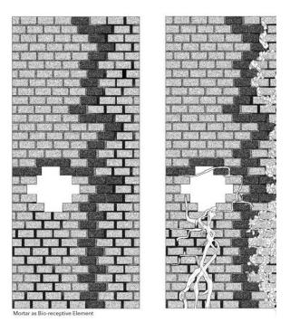
**Fig 3.** Mortar as bio-receptive element and Brick protrusion to control biological colonization (Aswin Senthil 2021) as part of Ecotone: The Sentient Ruins Studio, CEPT University, Tutored by Prof. Sonal Mithal
