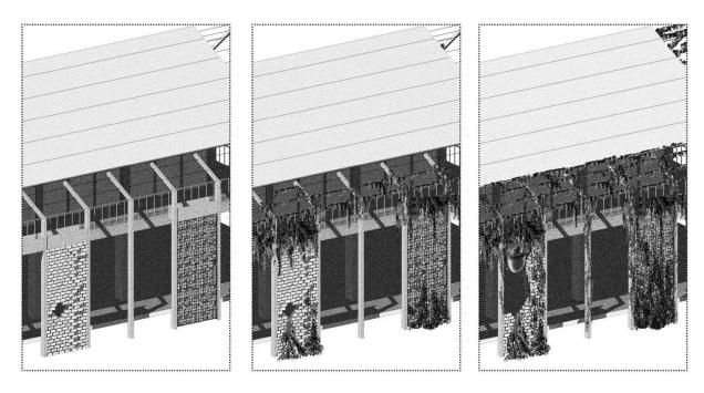
**Fig 4.** Mortar as bio-receptive element and Brick protrusion to control biological colonization (Aswin Senthil 2021) as part of Ecotone: The Sentient Ruins Studio, CEPT University, Tutored by Prof. Sonal Mithal
